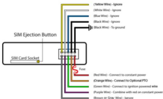
*Basic wiring diagram*
